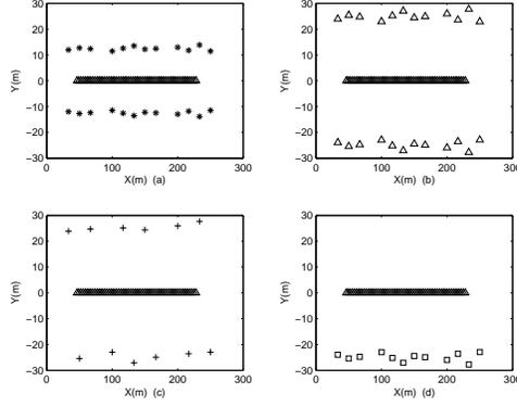
Fig. 1. Sensor Deployment, (a) dense sensor close to road, (b) dense sensor, (c) loose sensor located at two side, (d) loose sensor located at one side
