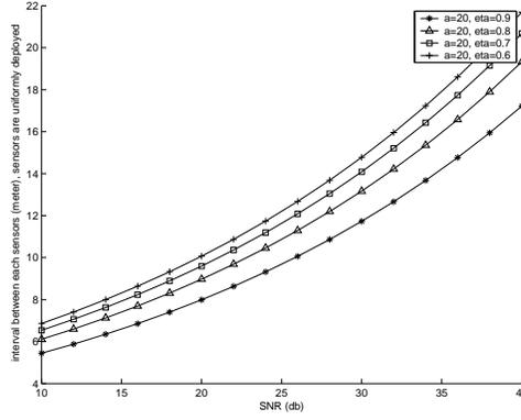
Fig. 4. relation between maximum sensor interval and SNR, the confidence level
