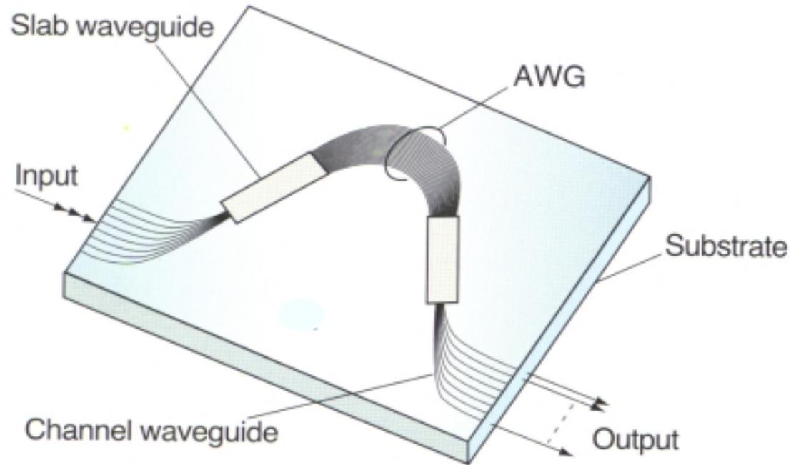
Waveguide pattern of AWG multi/demultiplexer chip
